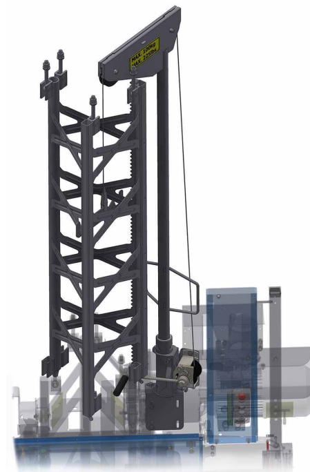
Fig. 69: Lifting, positioning of mast parts
